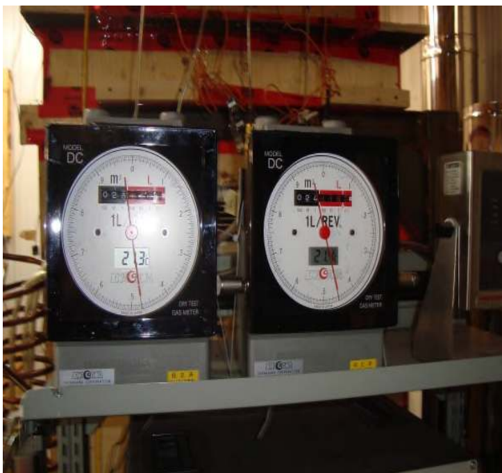
Picture 11: Dry gas meter
